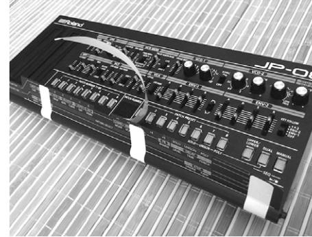
**Attention:** The adhesive strips (for temporary fixation) must **not come loose** during this time! In addition, make sure that the now-adhesive overlay does **not touch** the device in this step.
